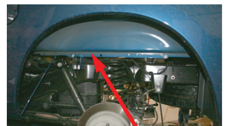
Plastic Wheel Well liner Removed
